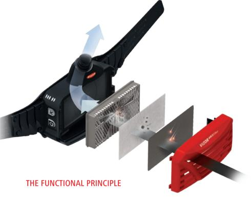
The fresh air system consists of a fresh air blower, interconnecting hose and carrying strap. The fresh air blower attached to the carrying strap filters up to 99.8% of welding fume particles out of the ambient air via a TH3 particle filter (highest possible classification) and directs the cleaned air directly into the Vizor Connect via the interconnecting hose. This represents an almost 100 percent improvement in terms of exposure to welding fume particles.
