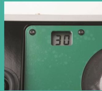
The grinding angle is shown in the digital readout.
