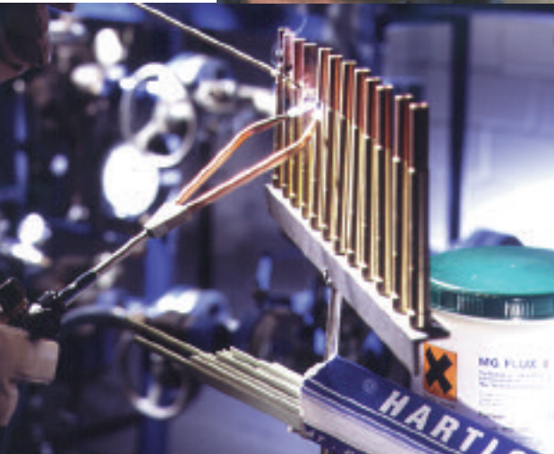
MINITHERM® brazing in industrial mass production.
