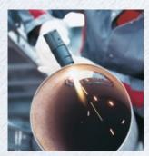
The drastic reduction in flying sparks means that much less subsequent cleaning and remachining is needed.
