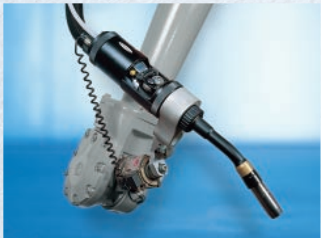
Robacta Drive with external wire guidance system: Inner liner can be changed very quickly, downtime is minimised.
