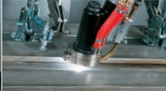
Automated plasma-keyhole welding of a longitudinal seam
