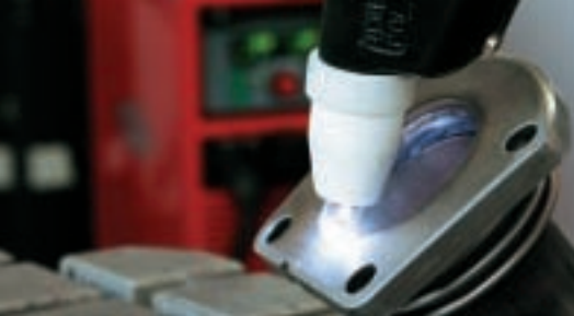
A flange-to-tube joint being soft-plasma welded
